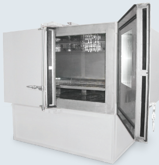
FBAR Front-to-Back with Reversible Air Flow
