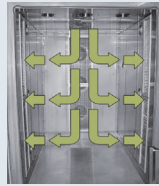
FBAR Front-to-Back with Reversible Air Flow
