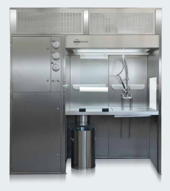
The WIBOjekt® workbench, type TGRJO, is designed in compliance with GMP and is suitable for installation in clean rooms. All system parts are designed in such a way that there is very little dead space and they are easy to clean. The system can be used in a versatile manner, such as for weighing, emptying and filling powders and liquids or dust-like products in the laboratory. Further application options are possible.
