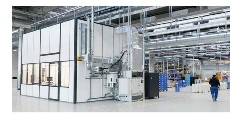
checks supplier's parts for dimensional accuracy. The second measuring room is concerned with quality assurance during and at the end of the in-house manufacturing process. "Some of the manufacturing tolerances to be measured are about one µ," says Jörn Winkler.
