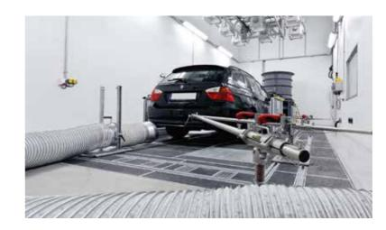
In addition, it permits sunlight simulation at up to 1000 W/m². On the test bench, an airstream blower creates wind with a velocity of up to 120 km/h, proportional to the simulated driving speed.
