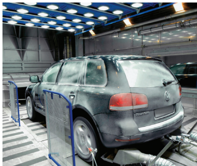
Full Vehicle Testing Combined Temperature/Humidity/Lights/Dyno
