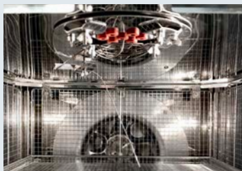
Moveable Product Sensor Measuring of product temperature
