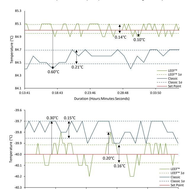
Figure 7: Temperature Fluctuation Comparison Between LEEF™ and Classic Refrigeration Systems
