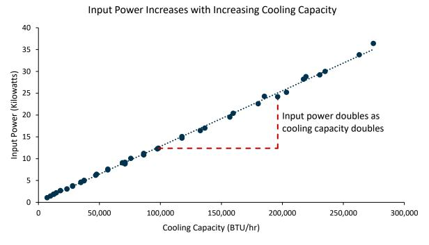
Figure 1: Relationship Between Input Power and Cooling Capacities<sup>1</sup>
