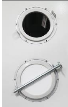
Figure 14: Port Plug Retention Bar
