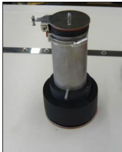
Figure 11: Venting Duct with Mechanical Check Valve
