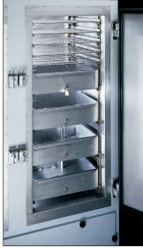
At left: Each of the large door accesses reveals a work area with an arrangement of removable stainless steel wire shelves and removable 6"-deep cement curing trays.
